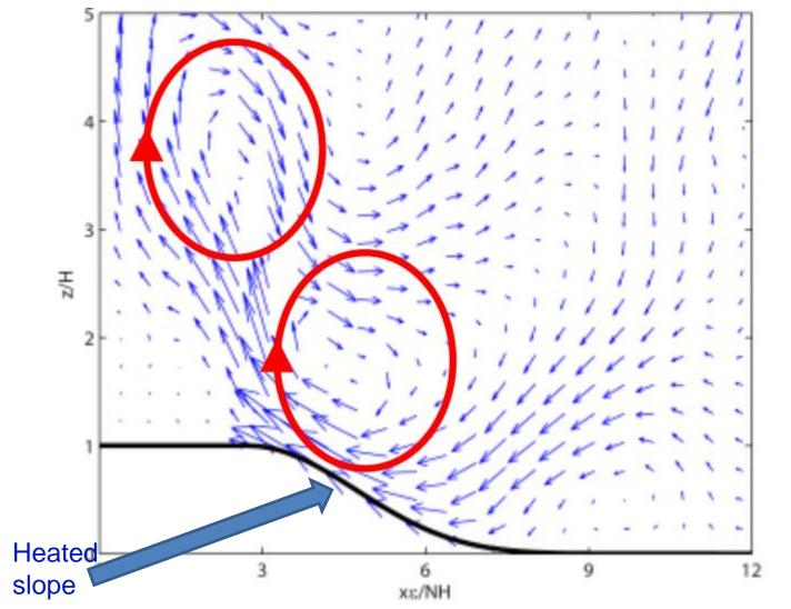
Two circulation cells along a heated slope simulated using a 2D model from Qian et al. (2012, JAS)
