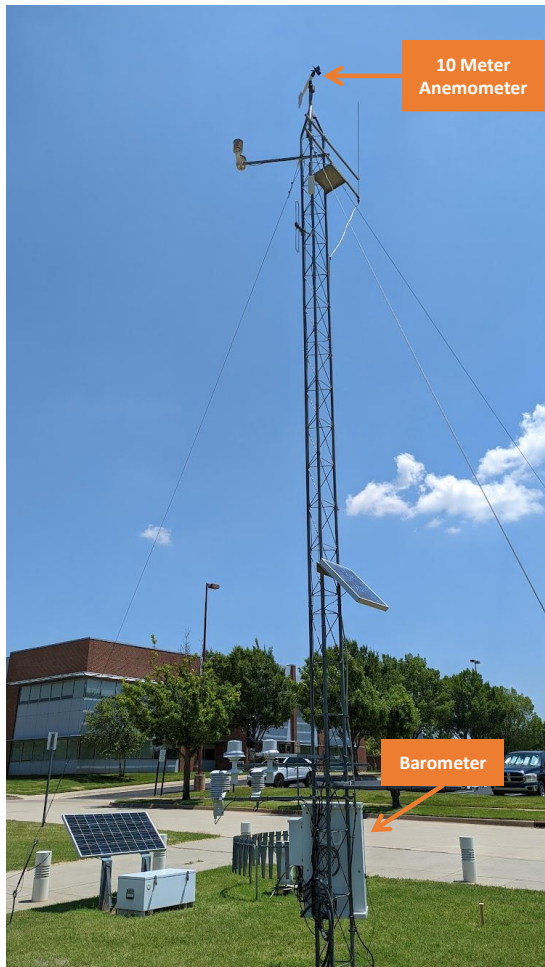
FIG. 3. Image of the Oklahoma Mesonet station at the National Weather Center in Norman, Oklahoma. Annotated in orange is the 10-meter anemometer and barometer locations on the station, with the 10-meter anemometer located at the top of the station, and the barometer located inside the metal instrument box affixed to the central beam of the station.
