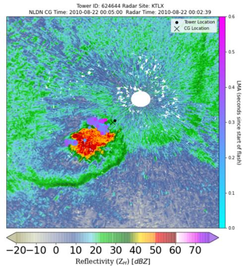
FIG. 6: LMA points of IC flash shown in Fig. 5 over  $0.5^\circ$  reflectivity from the KLTX radar at 0002 UTC on 22 Aug 2010.
