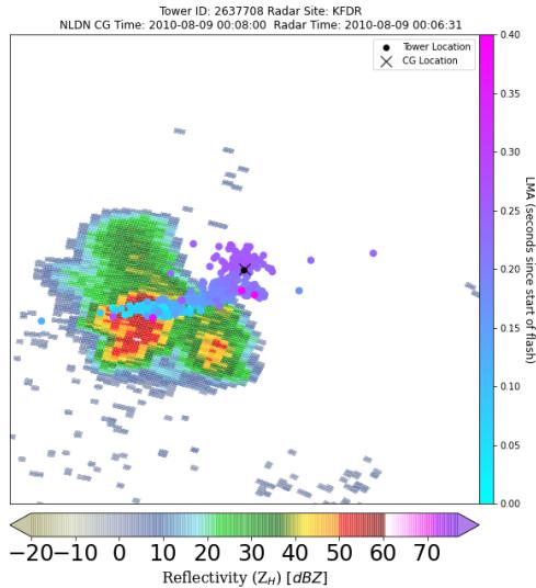
FIG. 4: LMA points (blue-to-pink with time) of CG flash shown in Fig. 3 over  $0.5^\circ$  reflectivity from KFDR WSR-88D radar at 0631 UTC.
