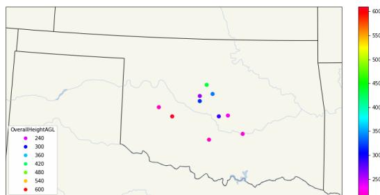
FIG. 1: Map of FCC communication towers across Oklahoma colored by height (AGL). Specific tower heights are listed in Table 1.
