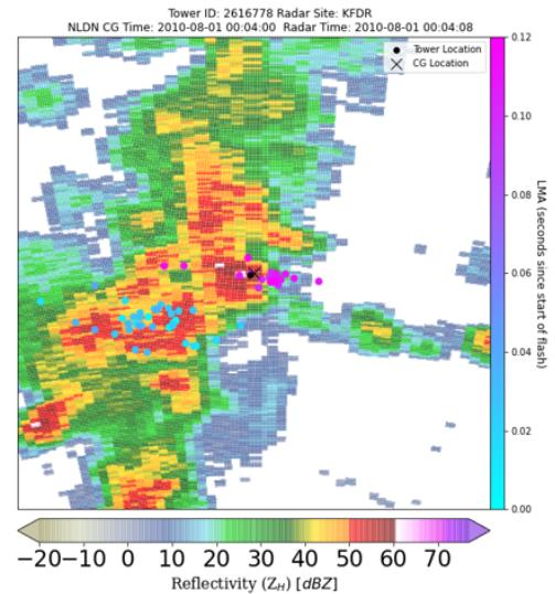
FIG. 8: LMA points of IC flash shown in Fig. 7 over  $0.5^\circ$  reflectivity from the KFDR radar at 0004 UTC on 1 Aug 2010.
